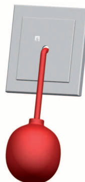
Pneumatic call unit with pneumatic switch element. Release through squeezing the red rubber ball on 2 m long clear plastic tube
